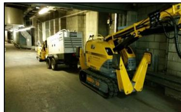
Operatives were manoeuvring two remote control Brokk demolition machines. The machines were towing (and being powered by) a diesel generator between the access point for the site and the platforms at the Waterloo International terminals.
