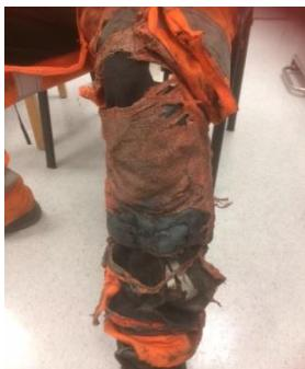
Whilst erecting Vortok fencing at Tunbridge Wells, an insulated shovel caused a short circuit between the conductor rail and running rail. This resulted in an electrical flash that burnt an operative's trouser leg.
