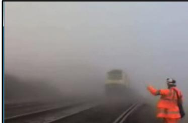
A train driver reported a near miss with a group of railway workers at Ladbroke Grove. The group were stood in the down main line CESS and were only seen at the last moment by the driver due to the weather conditions. The following control measures were not being implemented:
