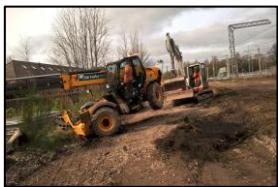
A lesson learned document has been released by colleagues at HS2 after a tele-handler was being misused on a site. It was reported that the boom was fully extended and the weight on the forks had caused the machine to become unstable. Further details can be found [here](#).
