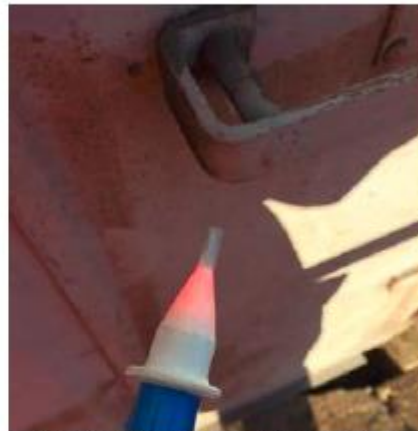
Volt-Stick showing the location cabinet is live during "Test before touch"
