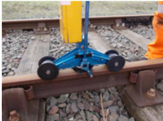
Figure 2 – Pre-use checking a trolley not fitted with rail wheel braking
