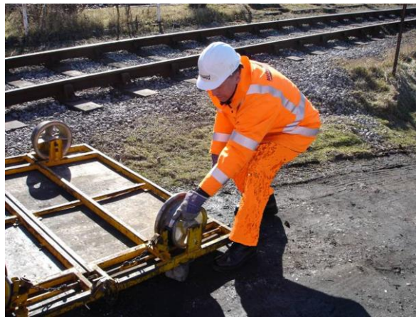
Figure 1 Undertaking a pre use brake test using one hand only
