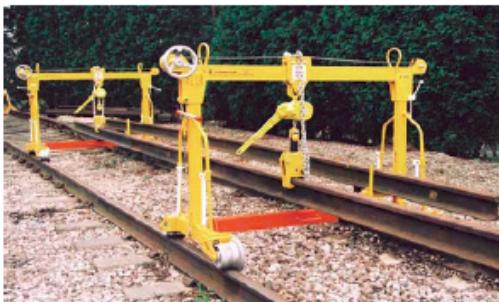
The Ironmen were being operated down a gradient which was up to 1 in 40, with the load for each pair being just short of 1 tonne. The rail head was contaminated with leaves and it was raining heavily at the time.
