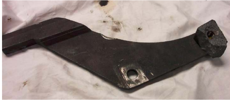
Ramp end with impact damage and bracket that hit passenger on the platform
