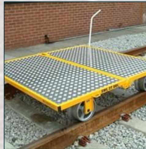
Link type trolley has a smaller loading area and weighs 47kg. Each link trolley can carry a UDL of 1000kg. Three link trolleys can be joined together, which can carry a UDL of 2000kg. This trolley can be used in gradients up to a maximum of **1 in 150**.
