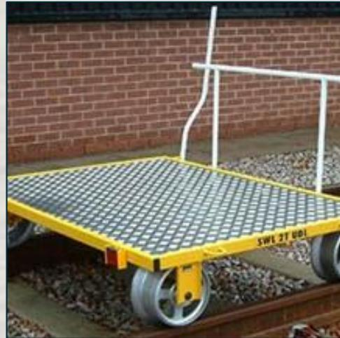
Type B trolley is in 2 parts and weighs 130kg. This has a larger loading platform than the type A trolley and can carry a UDL of 1000kg. This trolley can be used in gradients up to a maximum of **1 in 50** as per Handbook 10 GERT8000-HB10.
