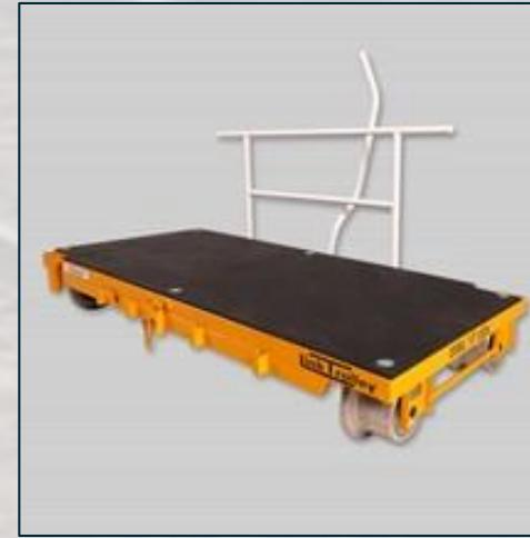
The gradient restriction of **1 in 150** applies to link type trolleys and manually propelled rails handlers (ironmen).
