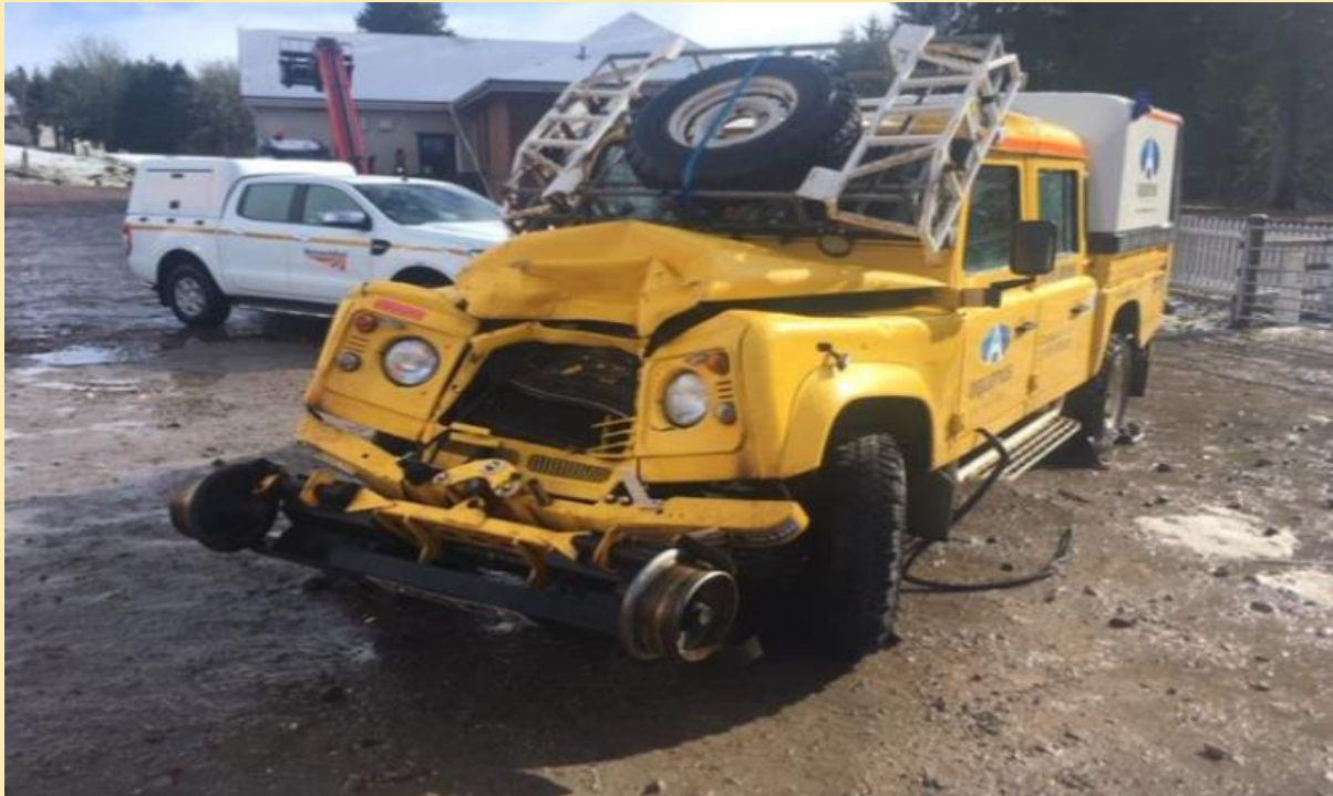
Damage resulting from collision between 2x OTP in Scotland in March 2019.
