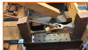
When the handle of the jack came up as a result of not being correctly clicked into position, a member of staff had his hand trapped between the handle and the opposite timber, sustaining a fracture to his right middle finger and laceration/bruising to his ring finger.
