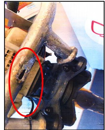
The Robel Hand Tamper with damage circled
